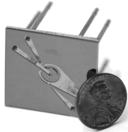
Fig. 9. Optical image showing an assembled turbopump device.
